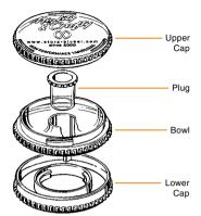
To fill the Filling Aid, remove the upper cap and fill the bowl incl. plug with ground plant material. Replace the upper cap and close it.
