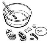
Manual cleaning of the disassembled Cooling Unit
