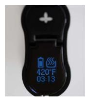
Toggle to the herb icon using the + and – buttons and press the power button twice in a row. Finally set your desired temperature and wait for about 30 seconds for the vaporizer to heat up.
