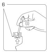
STEP 6: Use The Peak Dab Tool to place contents on the bottom surface of the bowl (not the side). (1) = Do not overfill. Dverfilling can damage your atomizer.
