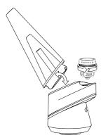
Preparation: Remove glass before unscrewing and re-inserting atomizer (do not overtighten, don't force it).
