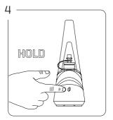
STEP 4: To power the device on/off, hold down the button for 3 seconds. () = Power down when finished to conserve battery life.
