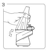
STEP 3: Align inlet hole on the front of the glass with atomizer. Carefully push the front of glass into the base, then the back.
