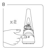
STEP 8: Double click to initiate heat-up. Press and hold button anytime to exit. Pulsing light indicates heat-up mode is active. ①\*See p. 11 for sesh mode.
