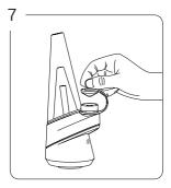
STEP 7: Place carb cap on top of atomizer. (i) = Protect your carb cap by using the tether provided.
