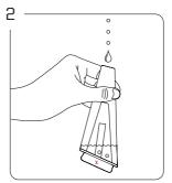
STEP 2: Fill glass with water just above the air-holes. Do not fill glass while attached to base. (1) = Water will damage base and atomizer! (1) = Do not overfill glass.
