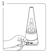
STEP 1: Fully charge device before first use. Device pulses white while charging, and turns off automatically when complete.
