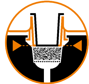
The lower rim of the Filling Aid must be above the top level of the plant material
