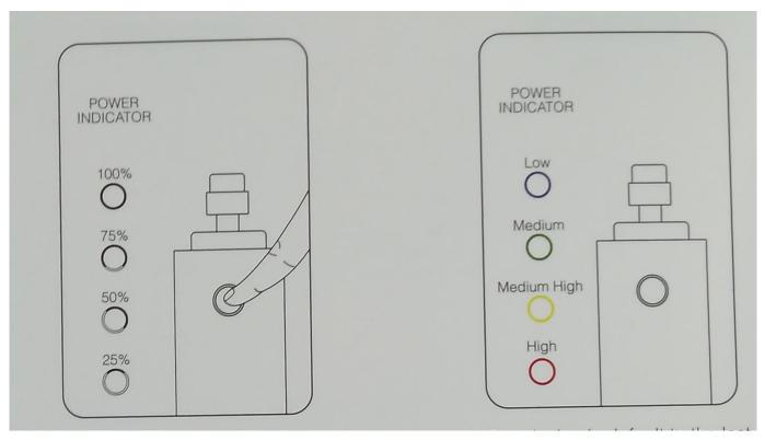
Press the power button five times quickly to turn the device on or off. The device enters standby when turned ON and the power indicator becomes solid and displays the battery charge level.
