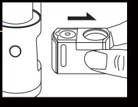
**3** Remove the magnetic bucket cover by pulling up.
