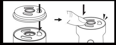
2 Screw the rechargeable battery clockwise into the NX base until tight, but do not over tighten.
